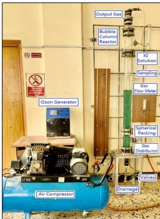
Figure 1. The experimental apparatus of packed bubble column reactor. Source: Author.
