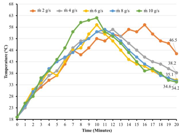
Figure 4. Profile temperature of the outlet from the coil heat exchanger. Source: Author.
