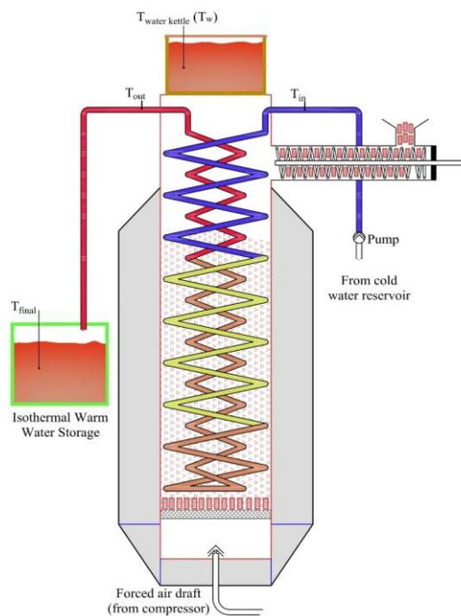
Figure 2. Schematic of experiment test by using time-to-boil (TTB) method. *Source: Author.*
