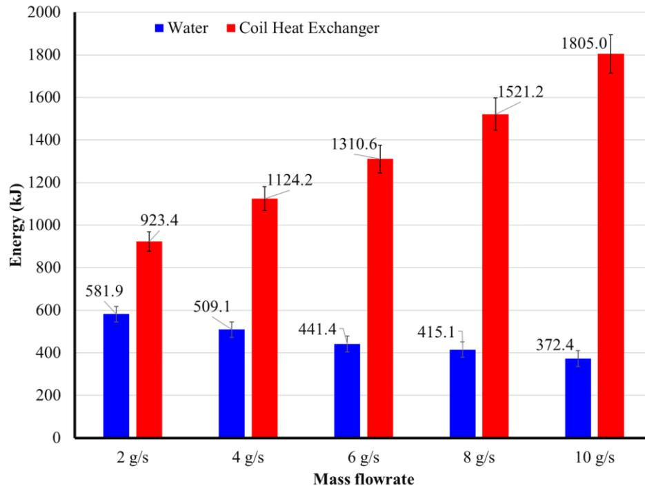
Figure 6. The absorbed heat energy for the water in the kettle and coil heat exchanger. *Source: Author.*
