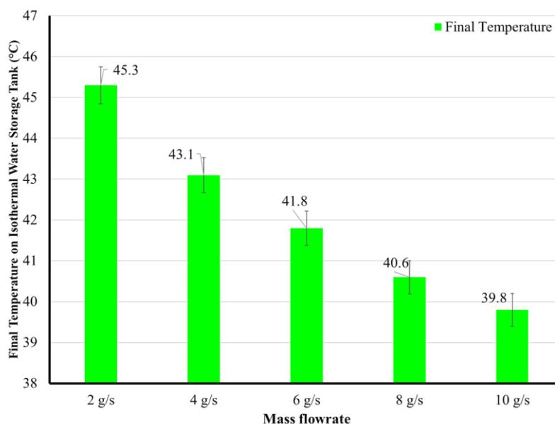
Figure 5. The final temperature on the isothermal warm water storage. Source: Author.
