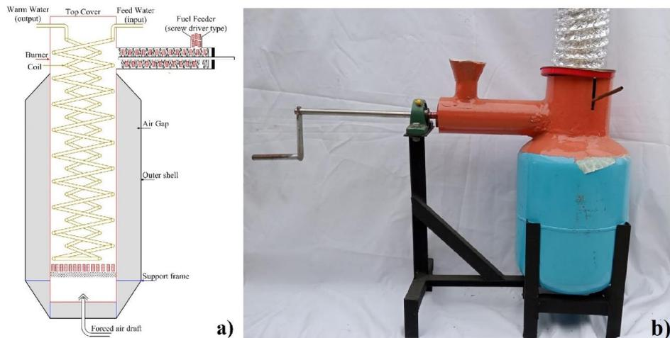
Figure 1. a) Schematic design for multipurpose biomass burner, b) Photograph of the prototype. *Source: Author.*
