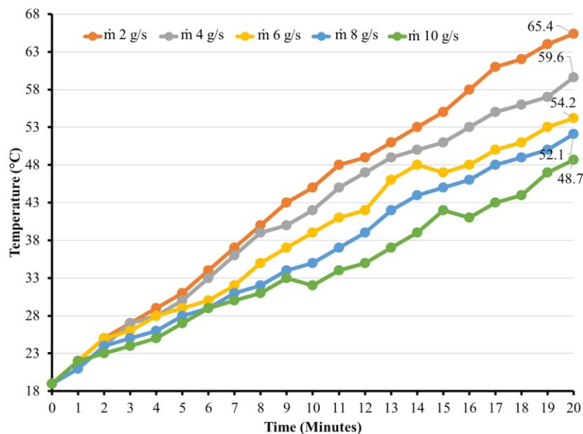
Figure 3. Profile temperature of the water inside the kettle ( $T_w$ ). Source: Author.
