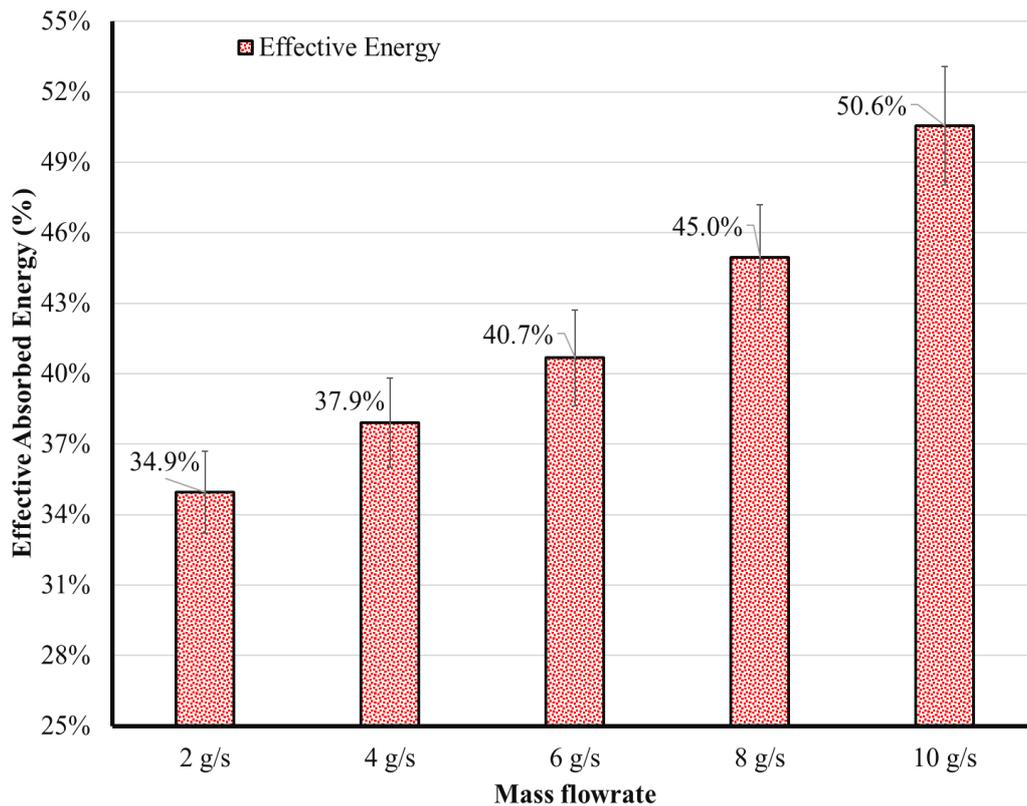
Figure 7. The ratio of effective energy absorbed by the water on the kettle and coil side. *Source: Author.*
