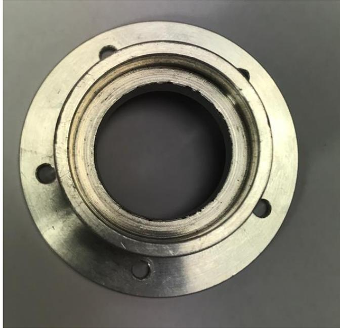
Fig. 3b. Inner part of aluminium hub
