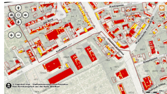
Photo: solar roof register City of Graz
