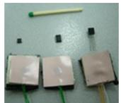
Figure 4. DS18B20 digital temperature sensors in flexible thermal conductive covers. Source: own materials.
