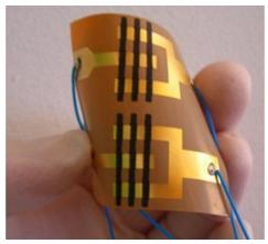
Figure 5. Flexible temperature sensor. Source: own materials.
