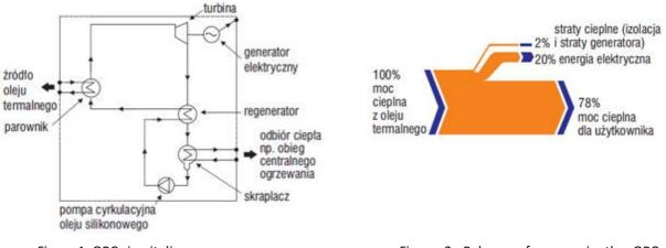
Figure 1. ORC circuit diagram.
