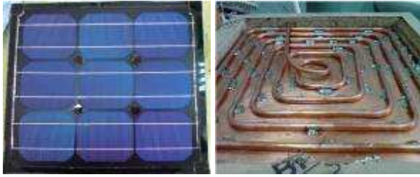
Fig.3. The realization of the solar hybrid system prototype: left – PV module, right- thermal collector.
