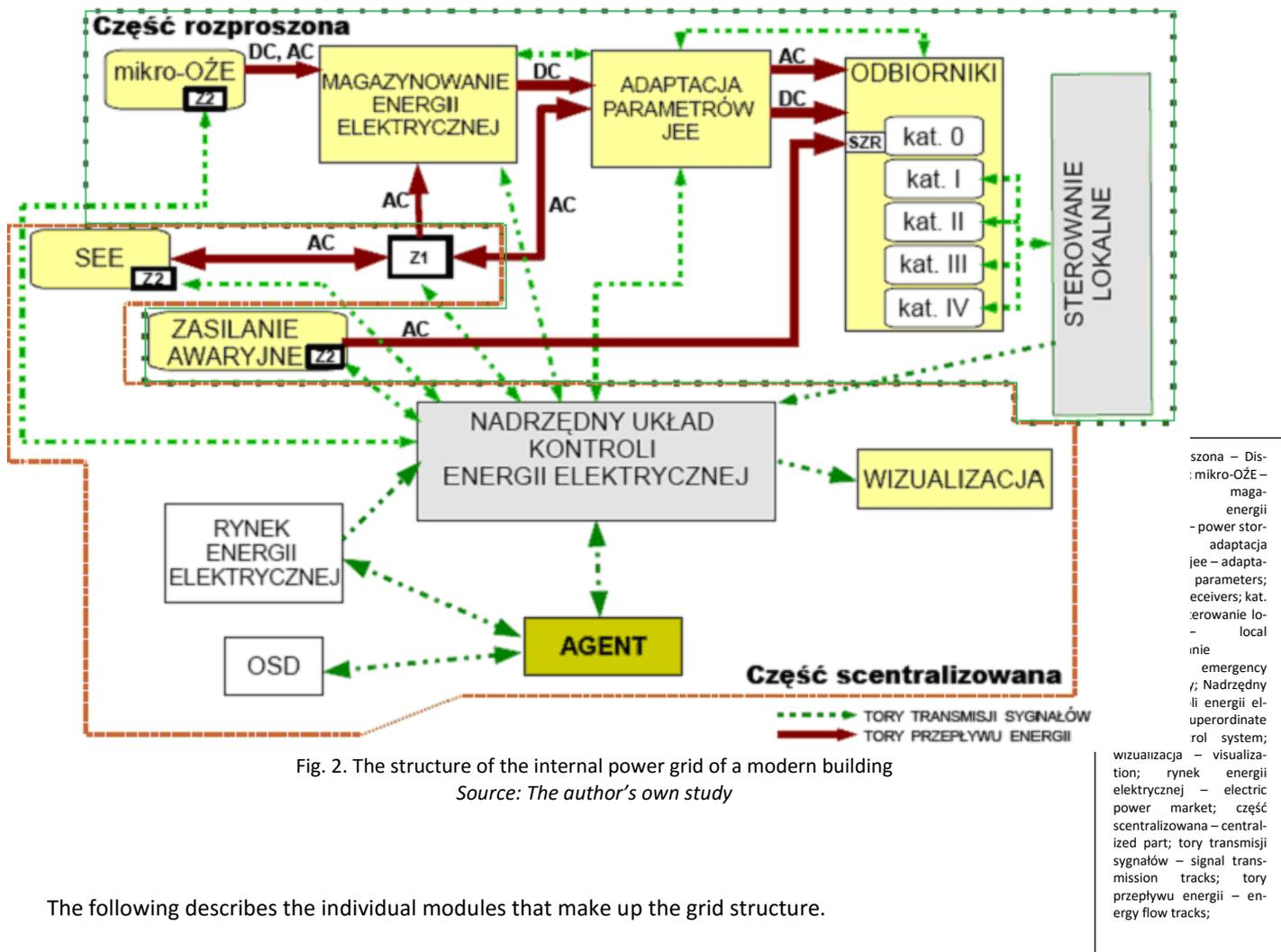
Fig. 2. The structure of the internal power grid of a modern building
