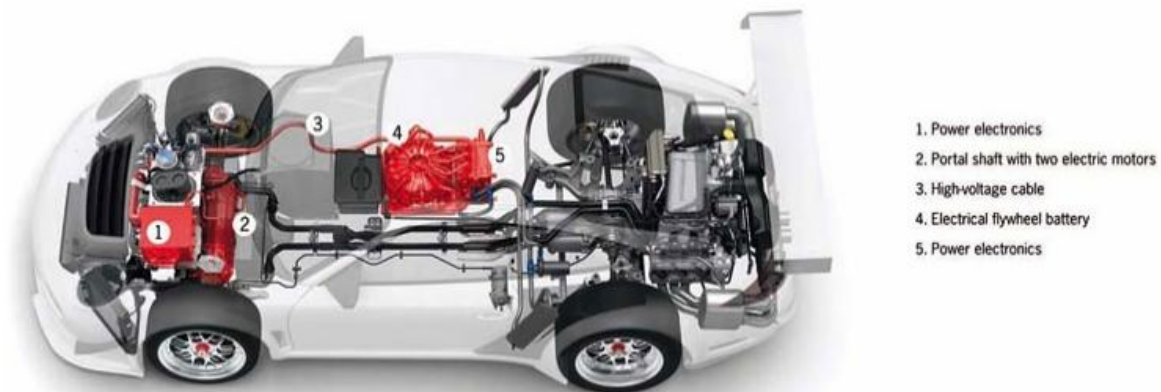
Fig. 3. Diagram of the electro-mechanical KERS system Source: [8]
