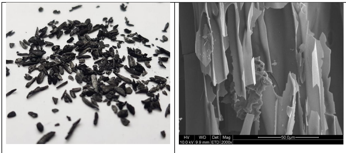
Fig. 2. Biochar particles image (left) and scanning electron microscopy (right, taken at Tel-Aviv University)
