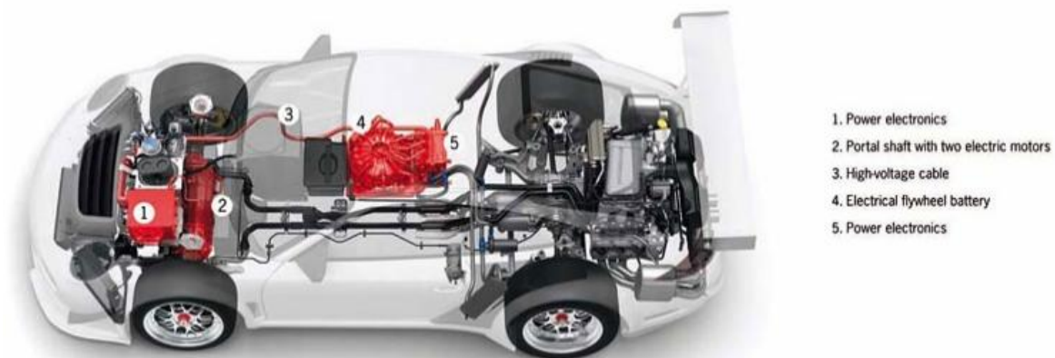
Fig. 3. Diagram of the electro-mechanical KERS system Source: [8]
