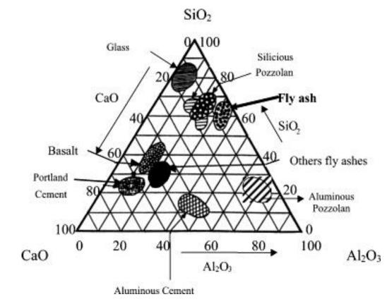
These mineral additions of PC have been in use for 4 decades. In principle, 2 types of mineral additions are used for direct mixing with Portland clinker or cement: ACTIVE, pozzolanic (natural and artificial pozzolans: thermally activated clays, fly ash, volcanic natural pozzolans, diatomite, silica fume) or hydraulically active additions (blast furnace slags), and **NON-ACTIVE**, crystalline fillers (siliceous or calcareous).
