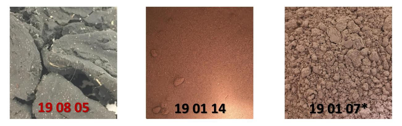
Originated during incineration fly ash (19 01 14) (9,0 Mg/d) and solid wastes from off-gas treatment (19 01 07\*) (0,5 Mg/d) are appropriately deposited at the "GOŚ-ŁODŹ" "Laguna" landfill site. Stabilized in this way sludge from treatment of urban waste water (19 08 05) (223 Mg/d) is deposited on the main square of the facility as non-toxic waste.
