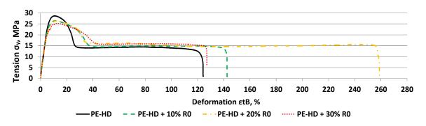
Fig. 3. Tensile curves of high density polyethylene and its mixtures with the addition of the grinding from the tank. Source: Author's
