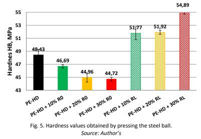
Basing on the research we can see that an increased amount of the HDPE waste causes an increase in hardness of the obtained PE-HD mixture. In case of the RO batch, an increase of the HDPE waste amount reduces the hardness. On the contrary, the RL batch shows the opposite behavior when the PE-HD waste is added.
