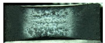
Fig. 8. The structure of breakthroughs of the original high-density polyethylene Source: Author's
