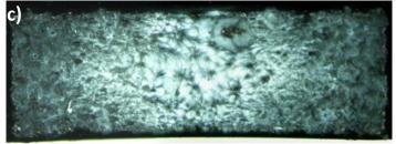
Fig. 9. The structure of breakthroughs of high density polyethylene with the addition of grinding originating from the fuel tank in an amount of: a) 10% b) 20% c) 30%. Source: Author's
