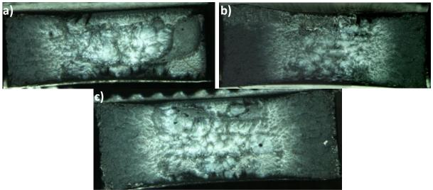
Fig. 9. The structure of breakthroughs of high density polyethylene originating from the production line in an amount of: a) 10% b) 20% c) 30%. Source: Author's
