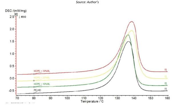
Fig. 7. DSC thermograms of the samples containing the grinding originating from the production line with respect to the unmodified PE-HD. Source: Author's
