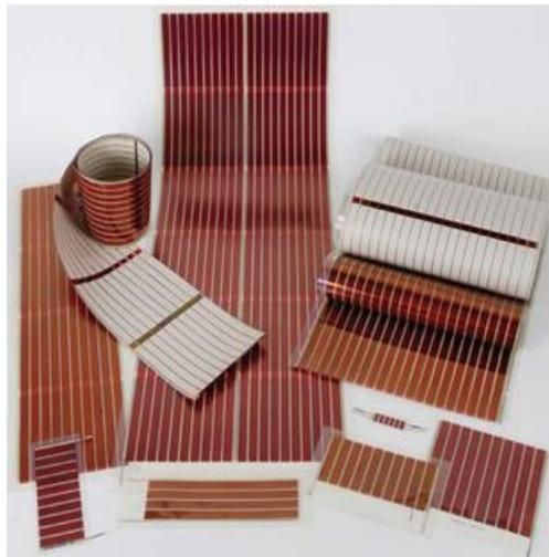
Figure 2. Flexible solar cells.
