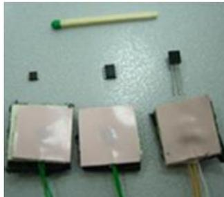
Figure 4. DS18B20 digital temperature sensors in flexible thermal conductive covers.
