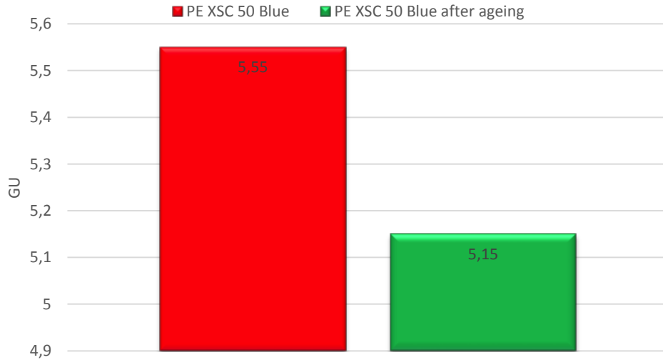
Fig. 9. Gloss investigations for polyethylene XSC 50 Blue before and after ageing Source: Author's
