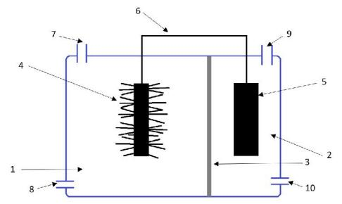
Fig 1. Scheme of typical two-chambered MFC. 1 – anodic chamber, 2 – cathodic chamber, 3 – membrane (PEM), 4 – anode, 5 – cathode, 6 –electric current, 7 – feed input, 8 – feed output, 9 – oxygen input, 10 – cathodic chamber output Source: Author's
