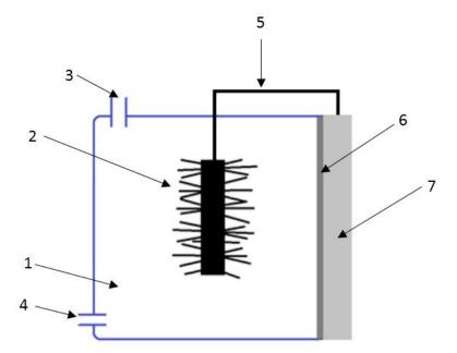
Fig 2. Scheme of one-chambered MFC. 1 – anodic chamber, 2 – anode, 3 – feed input, 4 – feed output, 5 -electric current, 6 -membrane (PEM), 7 – cathode Source: Author's
