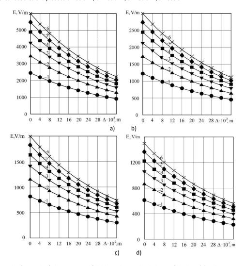
Fig 2. Magnitude of strength of electromagnetic field depending on the thickness of the layer ( $\Delta$ ) and microwave power (P) for mixture of finely-chopped greenery of spicy vegetables: 1-500 W; 2-1000 W; 3-1500 W; 4-2000 W; 5-2500 W; 6-3000 W, for surface area of a product: a-200 cm2; b-800 cm2; c-1800 cm2; c-1800 cm2
