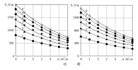
Fig. 1. Magnitude of strength of electromagnetic field depending on the thickness of the layer ( $\Delta$ ) and microwave power (P) for mixture of finely-chopped roots of spicy vegetables: 1-500 W; 2-1000 W; 3-1500 W; 4-2000 W; 5-2500 W; 6-3000 W, for surface area of a product: a-50 cm2; b-200 cm2; c-450 cm2; d-800 cm2.
