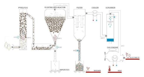
Fig. 5. Staged floating fixed bed gasification system by SynCraf. Source: SynCraft
