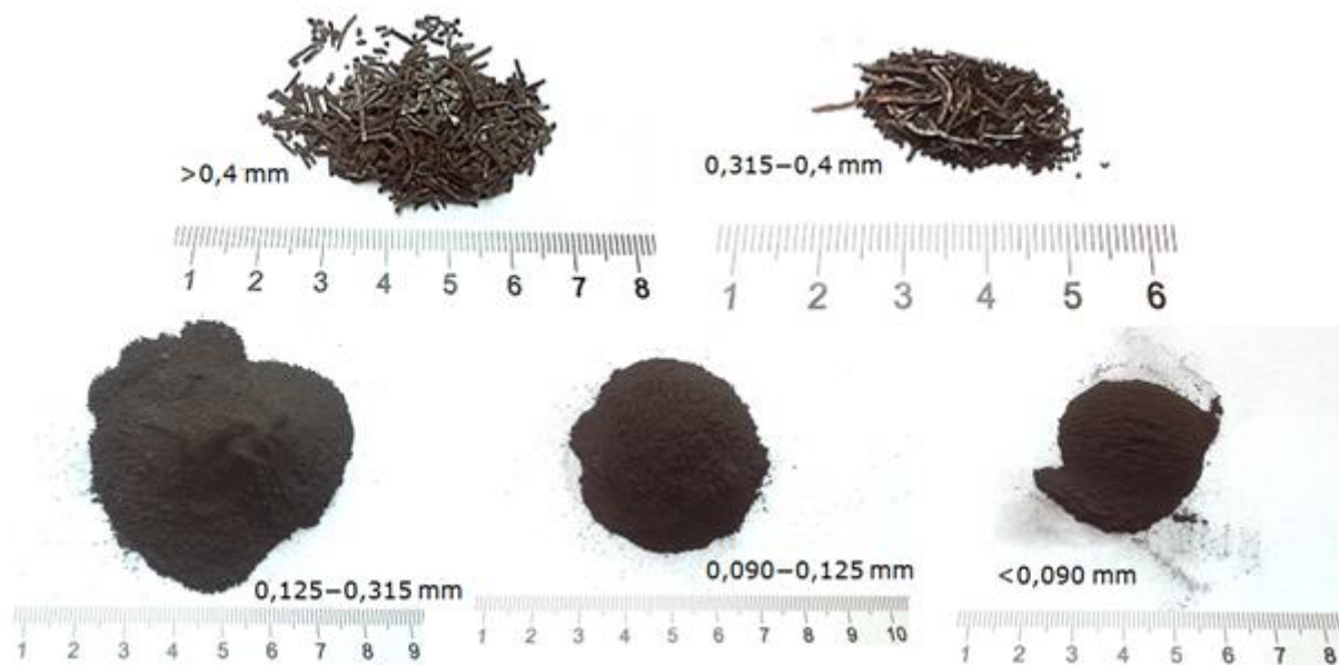
Figure 8. Fractions of pyrolyzed and ground tantalum capacitors
